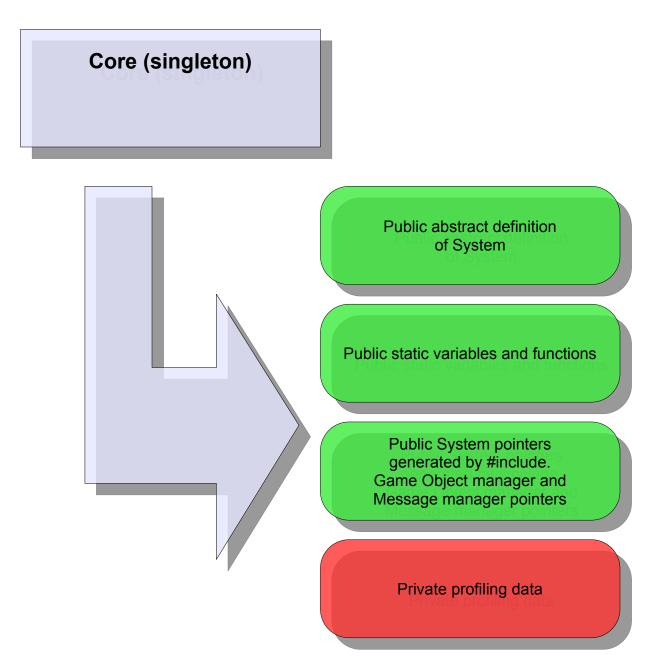
The Engine's Core is a singleton object which provides the main entry point into the engine. It contains 4 main points of functionality.
